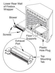
Figure 9 - Mounting Blower to Firebox
